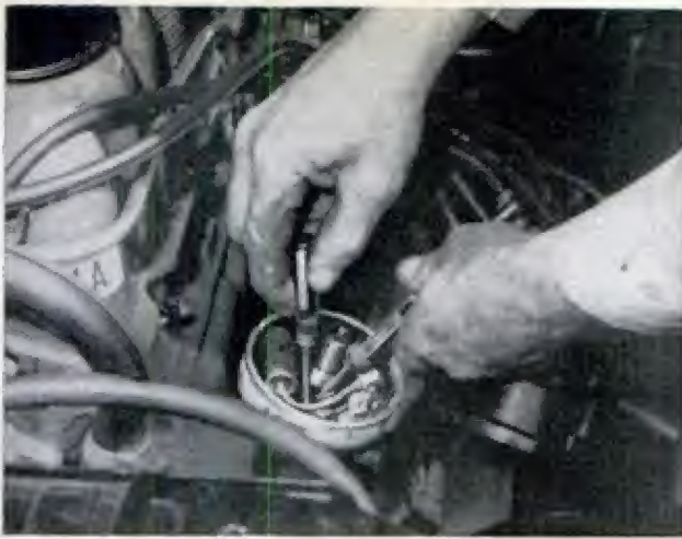
POINTS FEELER GAUGE is a small investment that will save you money. Keep it oiled to prevent rust
